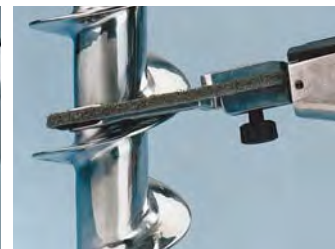
Clean and finish using non-woven nylon belts.
