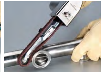
Clean and finish using non-woven nylon belts.
