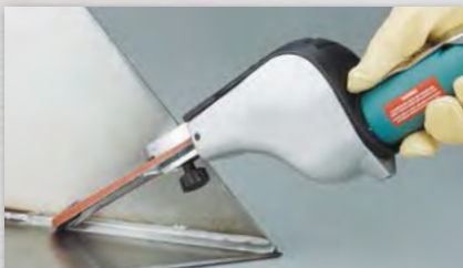
"THE ORIGINAL" DYNABRADE® Accepts over 35 interchangeable contact arms for hundreds of uses. 20,000 RPM.
