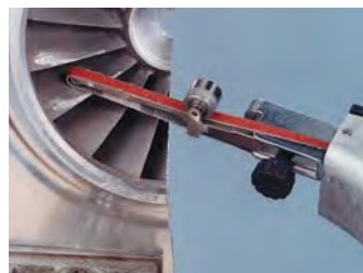
Efficiently rework turbine blades with specialized contact arm.
