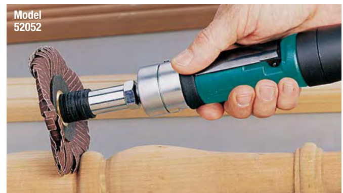
52052 Lightweight Dyninger with single arbor-mount star attached.
